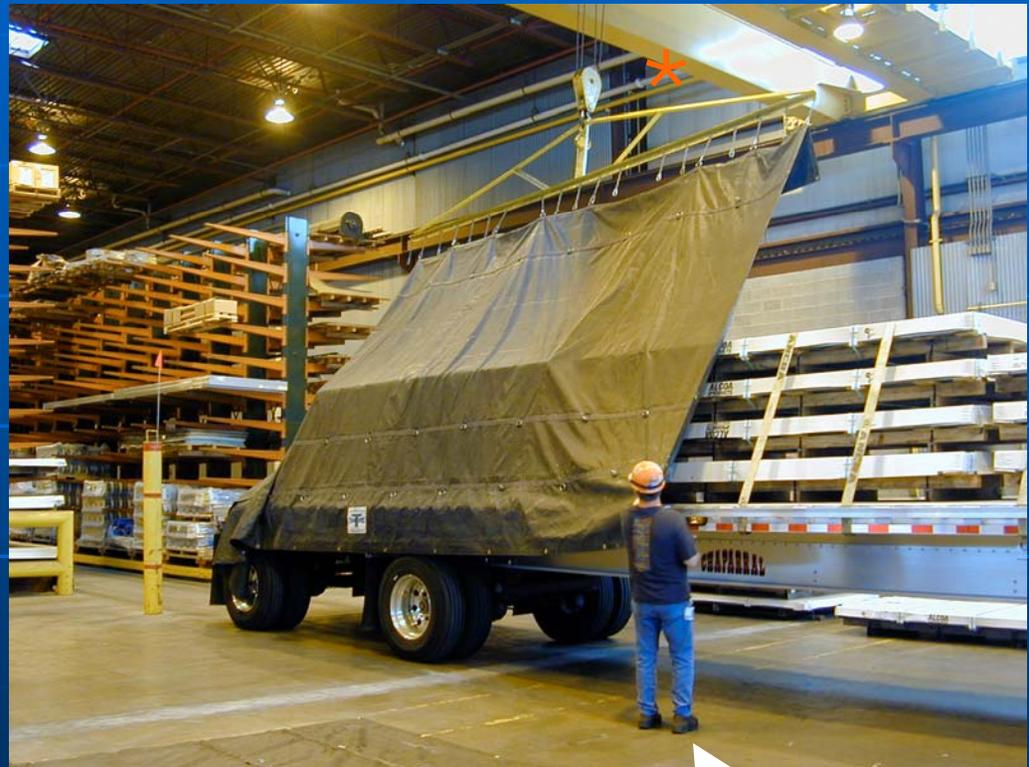
Request shipper fork lift operator to lift tarps or use Shippers Crane Spreader Bar (\*)
